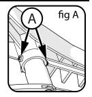
Ensure the seat is secure to the seat post and the seat bolt is tightened.
