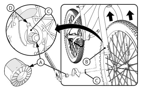
**NOTE:** Ensure wheel spins freely without contacting fork or fender.
