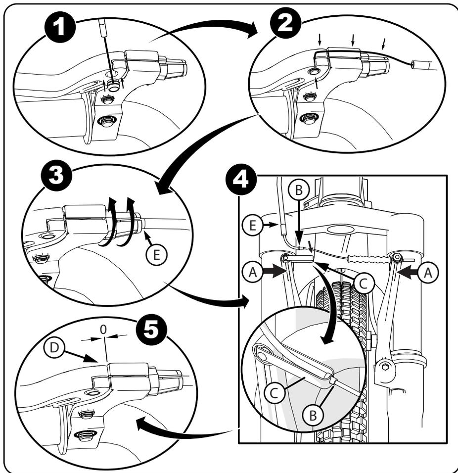
**Installing Front Brake Cable:**
