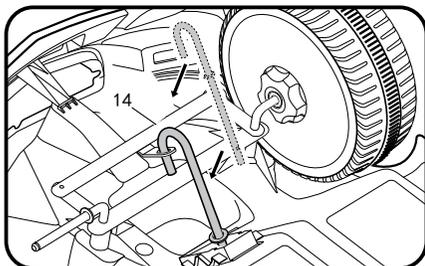
With the vehicle upside down, insert the long end of the J-shaped Steering Rod (part 14) into the body opening so that short end fits into the axle slot as shown.
