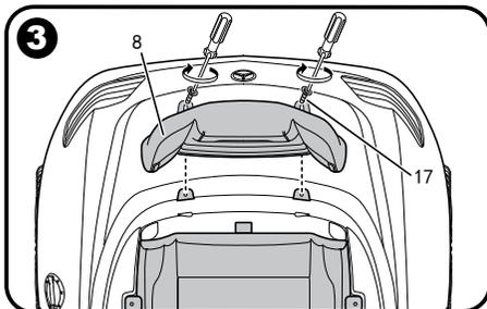
Insert the backrest (part 8) into place as shown and install the backrest screws (part 17) securely.
