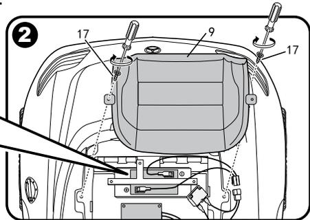
After the power supply is installed, put the seat (part 9) into the assigned location, and fix it with seat screw (part 17).
