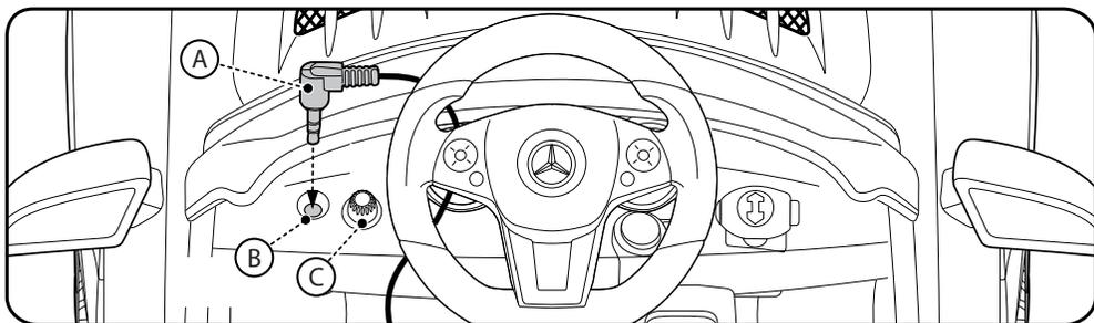
Insert the MP3 Plug (A) into the Socket on the instrument panel (B). Adjust volume by turning the Volume Knob (C) (next to the MP3 Socket).
