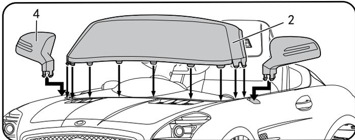
Install the windshield (part 2) and rearview mirrors (part 4) by inserting the tabs into the vehicle slots as shown. Press tabs in until a “snap” is heard.
