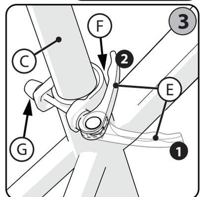
**⚠ WARNING:** You must use strong force to move the quick release lever securely to the “CLOSE” position **2**. This ensures that the seat does not move during normal operation.
