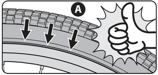
**⚠ WARNING:** Do not ride or sit on the unit if a tire is under inflated. This can damage the tire, inner tube and rim.
