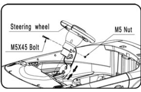
**NOTE:** Hold Steering Shaft from underneath while installing Steering Wheel.
