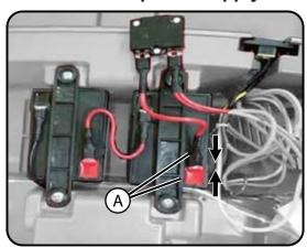
Attach the Power Connector to Battery Terminal (A) as shown firmly and securely.
