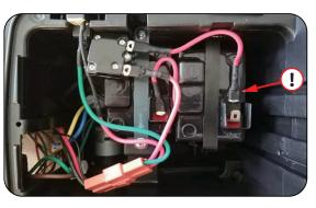
With Seat removed, firmly connect Power Connector to the Battery as shown.
